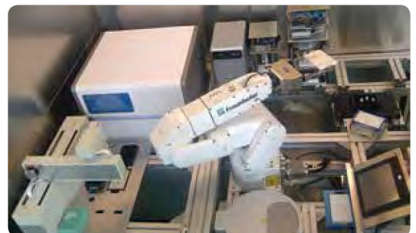
Automation cell, showing the 4LAB™, 4s3™ and De-Framer fully integrated
